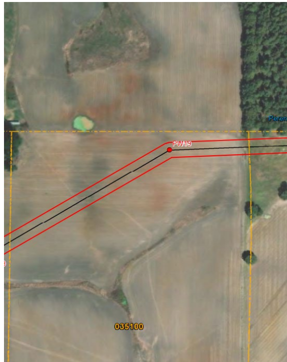
Proposed transmission line tower location on subject property.
