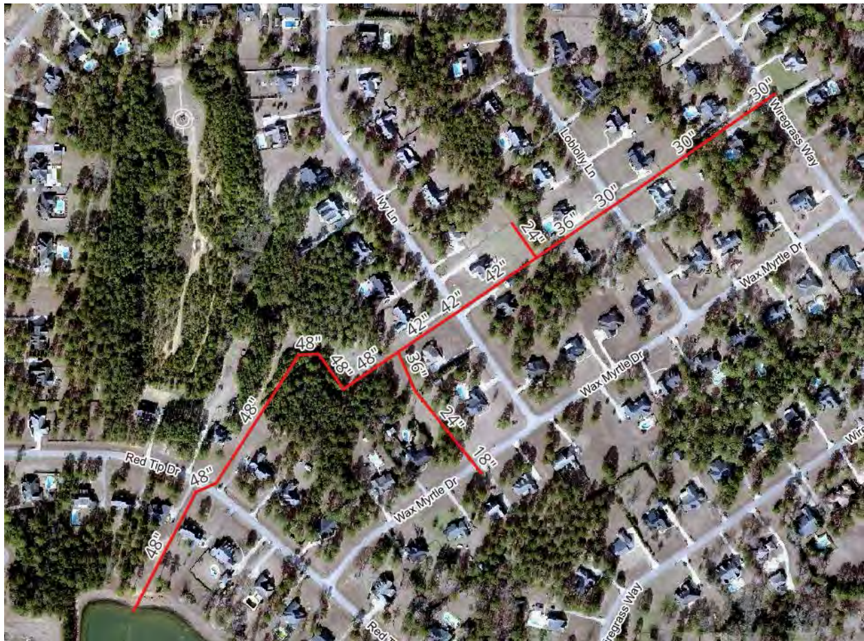
Figure 5 – Existing Pipe Network
